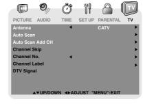
Use the ▲ / ▼ button to select Antenna, then press the ◀ / ▶ button to select Air or CATV.
